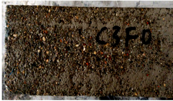
Fig. 4. 100 freeze-thaw cycles picture of damage in laboratory
